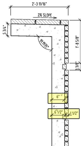
The existing panels weight in at 36 thousand pounds apiece. They impart all of their weight onto the exterior columns, which are then needed to be sized up in order to resist the additional force. It was proposed from the start of this project that the panels were needlessly heavy and could be thinned in some way to achieve better economy of materials and to reduce the forces on the superstructure.
