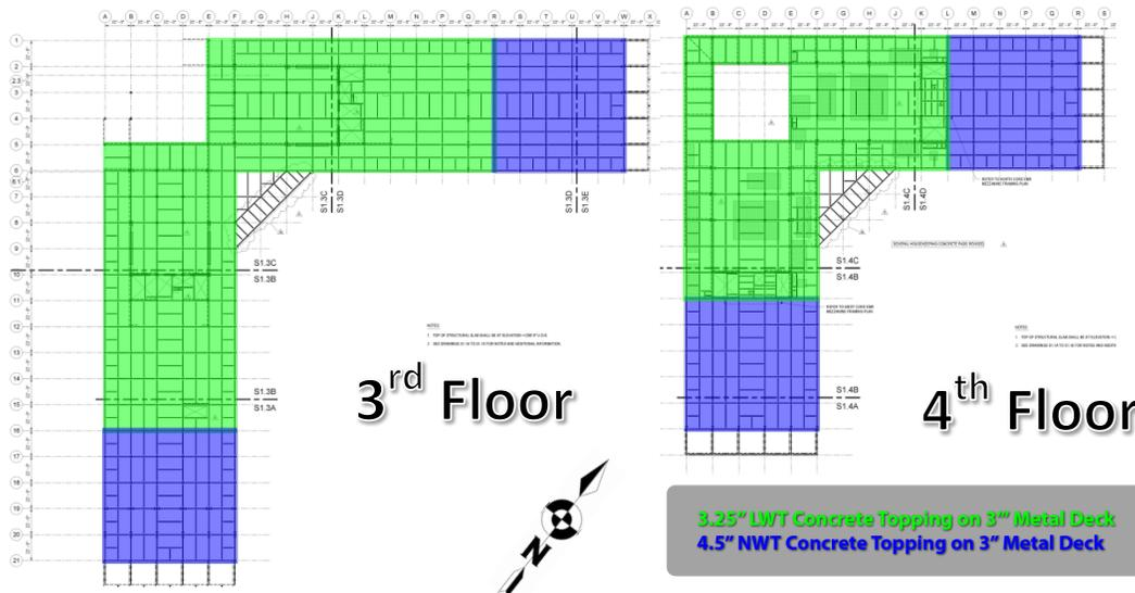
Figure 5.1: Plan View of the Third Floor
