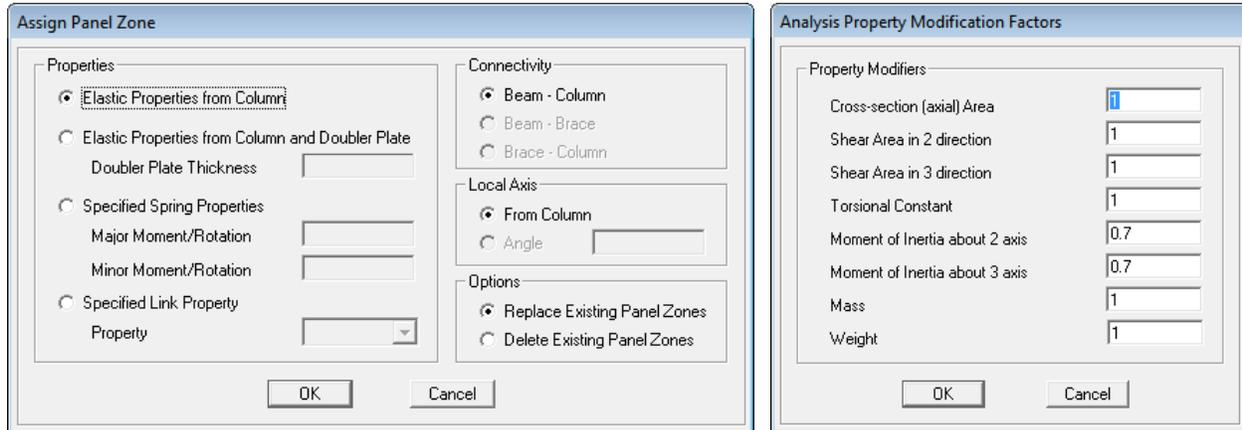
Figure 5.28: ETABS Torsional Irregularity Property Modifiers
