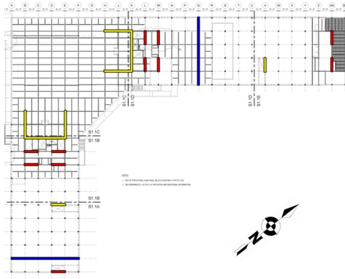
Figure 5.267: Plan of Lateral Elements
