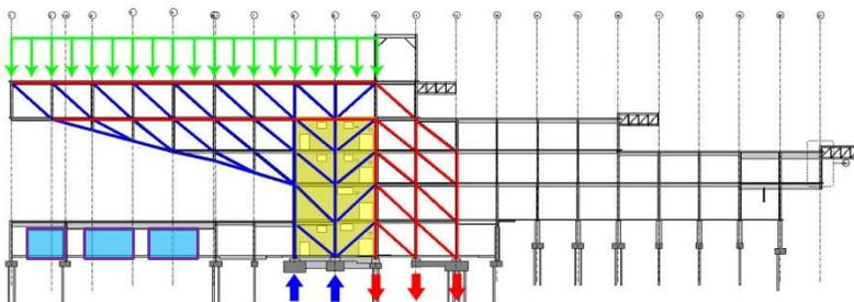
Figure 5.18: Existing Cantilever - Distribution of Forces
